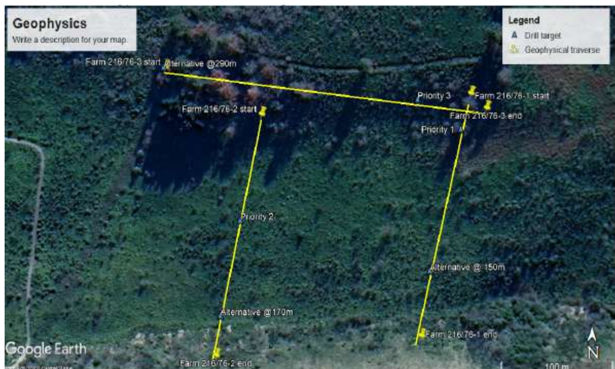
Figure 8 Planned Boreholes are close to the Northern border and far from the proposed Main Residence on the Southeast border. Ref Proposed Locations of the Boreholes - Appendix D3 & D10 Geotechnical Report - Page 31
