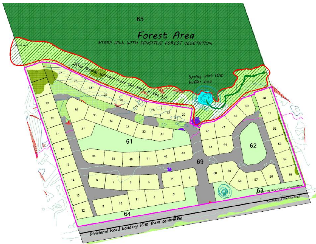
Figure 3. Preferred lower density development (January 2025). This SDP has been modified to pull Unit 50 back from the wildlife corridor which was recommended in a previous version of this report.
